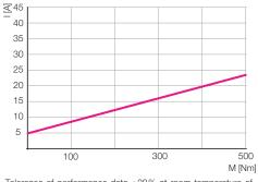
Tolerance of performance data  $\pm 20\,\%$  at room temperature of  $20\,^{\circ}\text{C}$  and run-in mode
