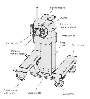
Rotating module mounted on lifting module Shop-Floor (available on request)
